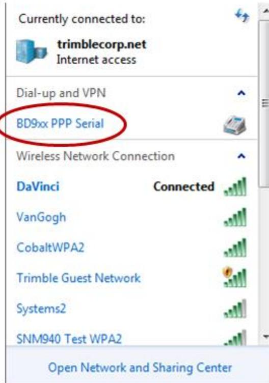
32. Connect the receiver to the computer at COM1 using a null modem serial cable. Click **Dial**. (No user name and password is required.)
